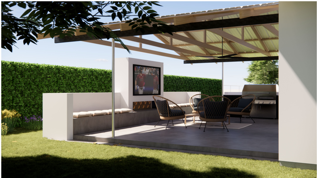
Image 3: Proposed covered patio and feature wall. Slim structural columns are placed at the 16' setback line.
