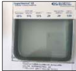
GLASS MANUFACTURER: GUARDIAN SUNGUARD COLOR: SUPERNEUTRAL 68 TYPE: LIGHT GRAY-SOLAR TINTED IN A CLEAR ANODIZED FRAME VIABLE LIGHT: TRANSMITTANCE: 68% REFLECT OUT: 11% REFLECT IN: 12% U-VALUE: 0.29 SHGC: 0.38 LIGHT TO SG: 1.80
