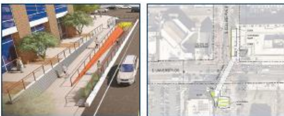
OPTION 2B: SINGLE TUNNEL, EAST SIDE OF COLLEGE AVENUE REALIGNMENT OF COLLEGE AVENUE REQUIRED
