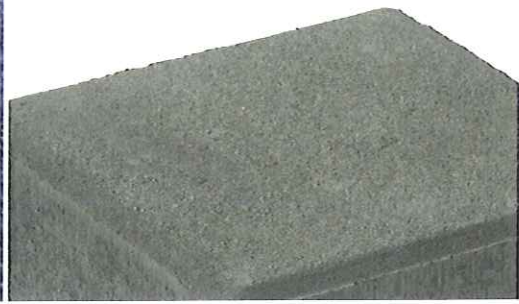
charcoal accent-concrete paver at parking
