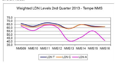
Ldn A decreases with the distance to the airport's runways. The monitored standard deviations are naturally higher for the monitors located at sites in Tempe located outside the downtown area south of the riverbed, where the distances to the aircraft as one of the sources of noise in the local environment are greater.
