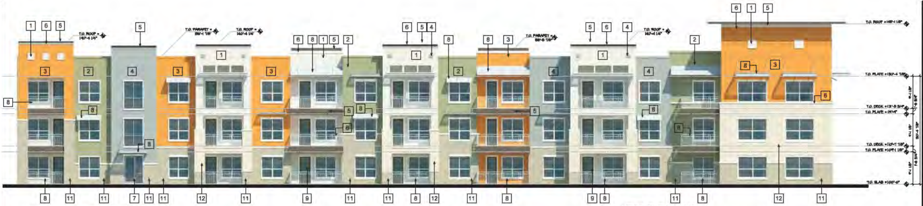
03 WEST ELEVATION BUILDING D' SCALE: 1/8"=1'-0"
