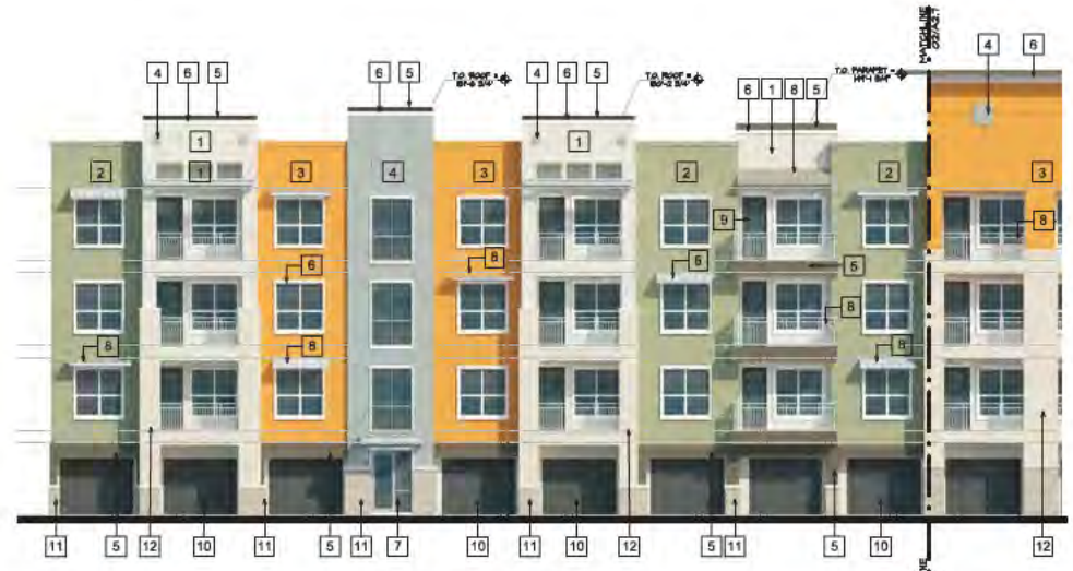
02 EAST ELEVATION BUILDING 'A' SCALE: 1/8"=1'-0"
