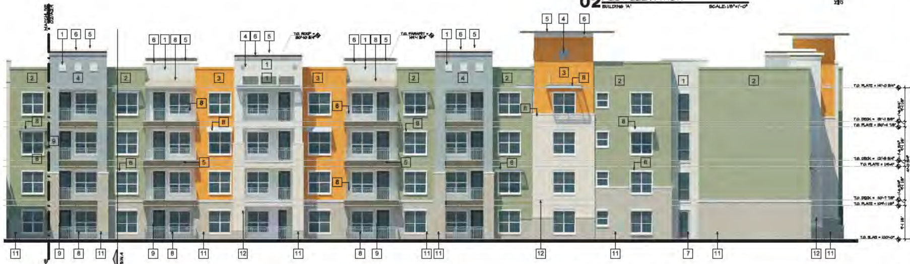
01 WEST ELEVATION BUILDING 'A' SCALE: 1/8"=1'-0"
