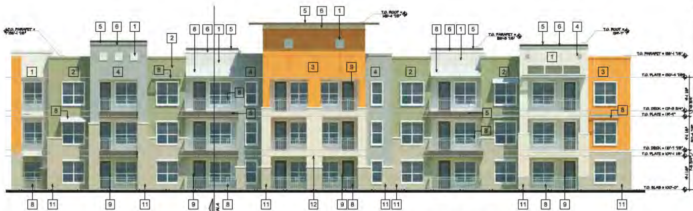
03 WEST COURTYARD ELEVATION BUILDING 'D' SCALE: 1/8"=1'-0"
