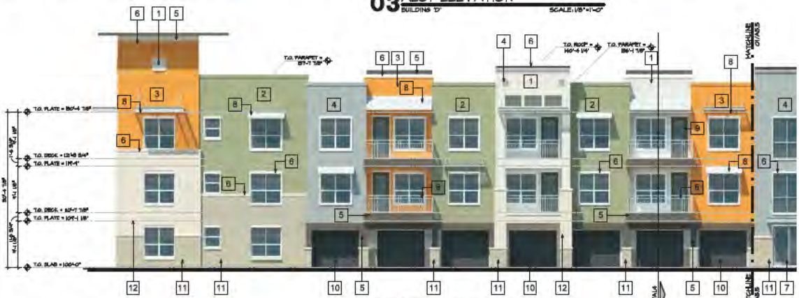
02 SOUTH ELEVATION BUILDING D' SCALE: 1/8"=1'-0"
