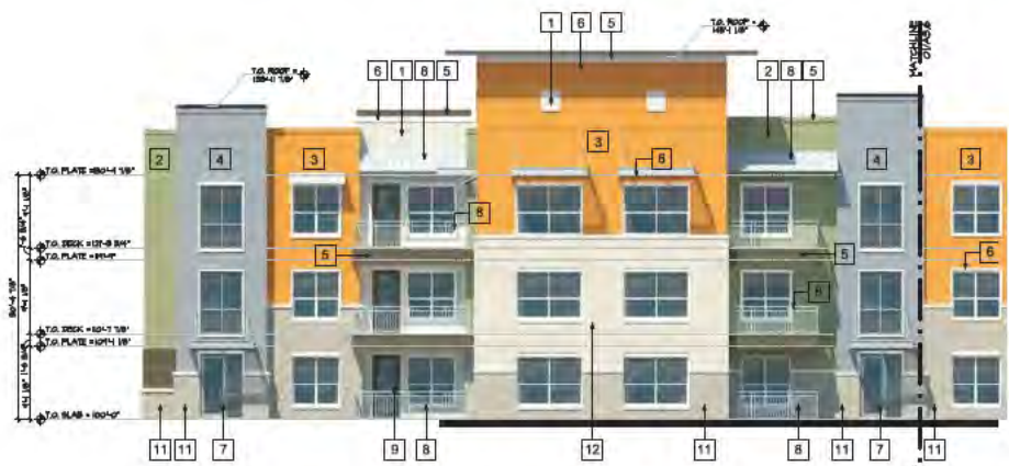
02 WEST ELEVATION BUILDING 5 SCALE: 1/8"=1'-0"
