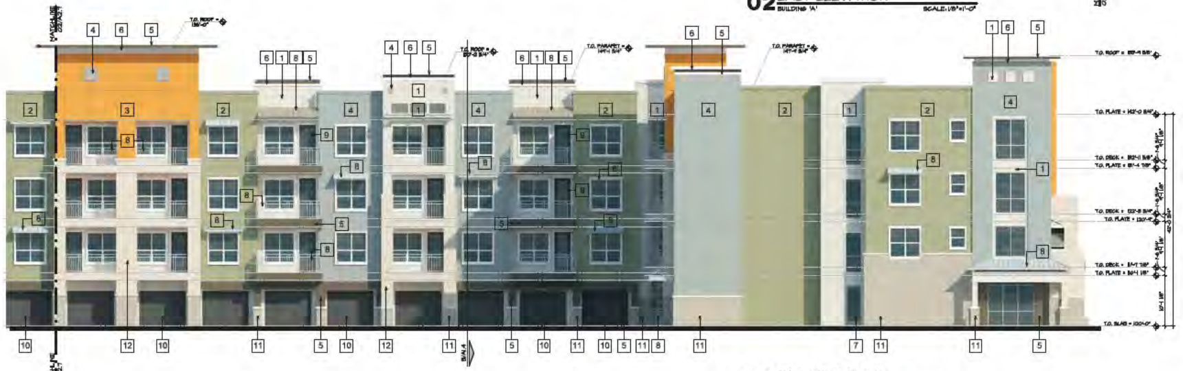
01 EAST ELEVATION BUILDING 'A' SCALE: 1/8"=1'-0"
