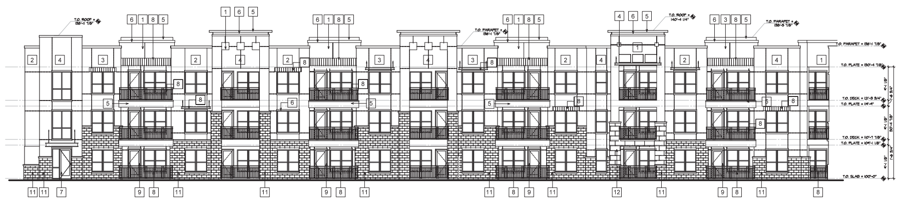
02 WEST COURTYARD ELEVATION BUILDING B SCALE: 1/8"=1'-0"
