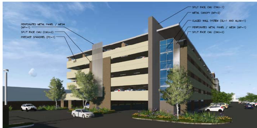
NORTH WEST ELEVATION TOC SCALE: NONE
