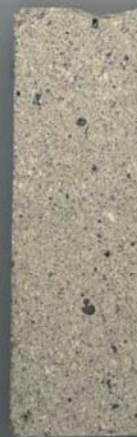
elevator run: mid grey cast-in-place concrete
