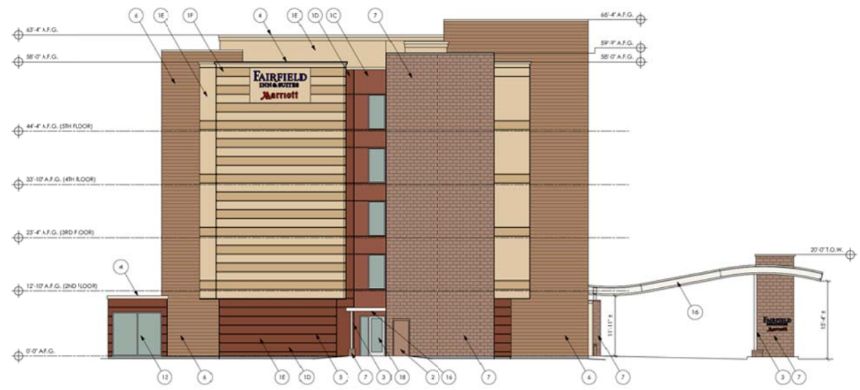
2 LEFT (SOUTHWEST) BUILDING ELEVATION SCALE: 1/8" = 1'-0"
