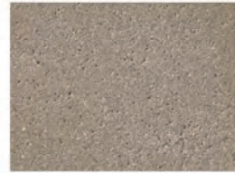
INTEGRAL COLORED CONCRETE FINISH: SANDBLAST
