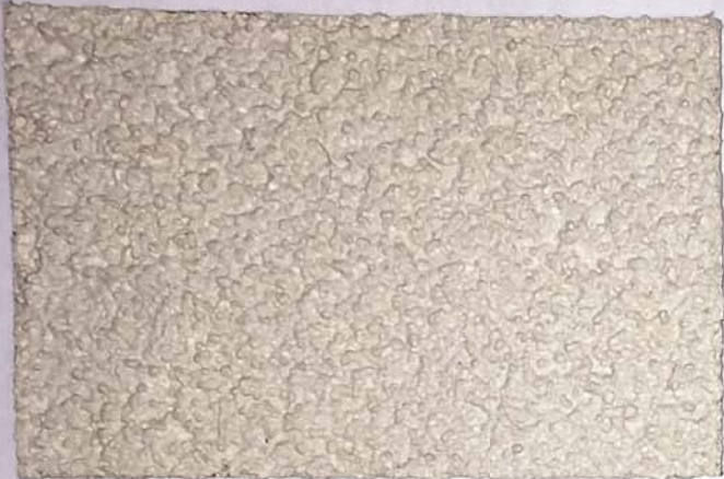
EIFS ABOVE WAINSCOT AT KIOSK STO MEDIUM FINISH SHERWIN WILLIAMS, SW7531 "CANVAS TAN" MATCH STORE COLOR LRV < 75%
