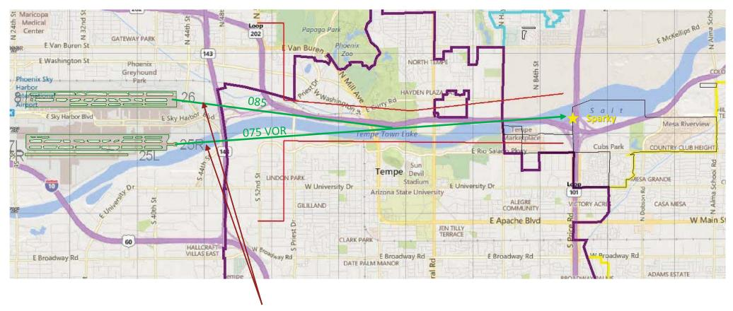
Headings off the center and north runways in place when the IGA was made and until the airport expanded with the third (south) runway.
