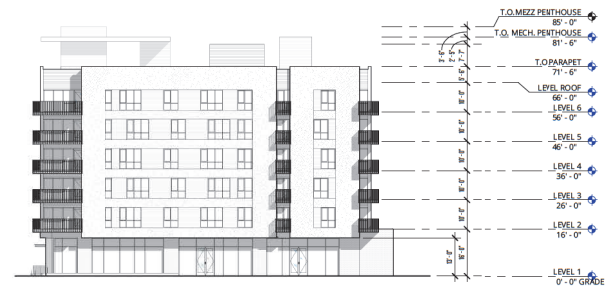
3 DPR - SOUTH ELEVATION W/ SHADOWS 1" = 20'-0"
