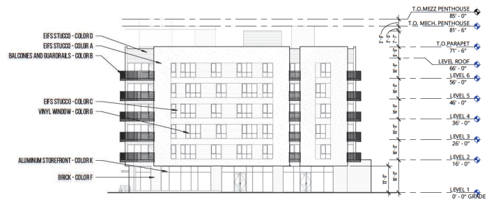
3 DPR - SOUTH ELEVATION 1" = 20'-0"
