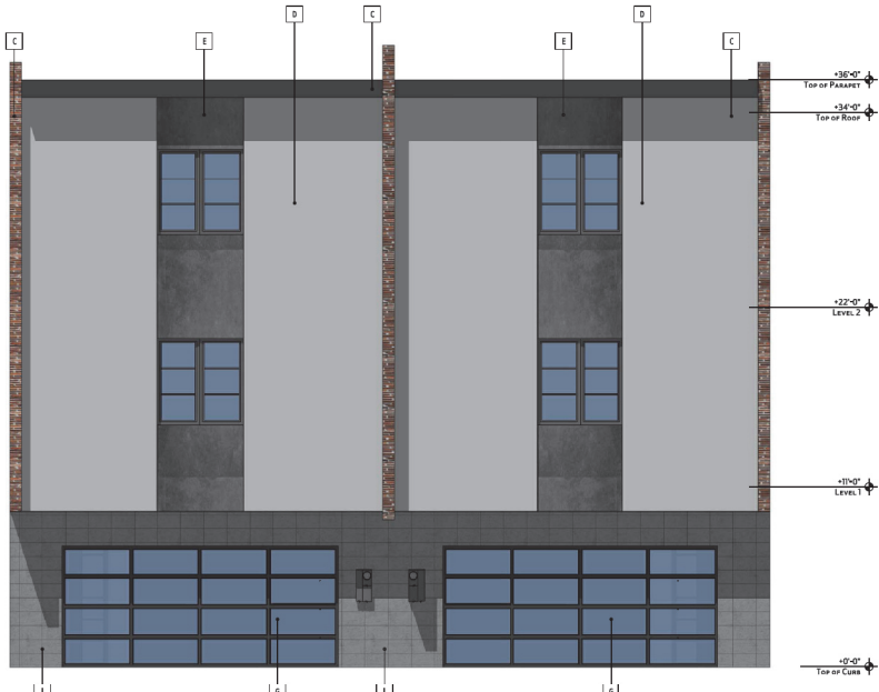
3 BUILDING B NORTH ELEVATION SCALE: 1/4"=1'-0"
