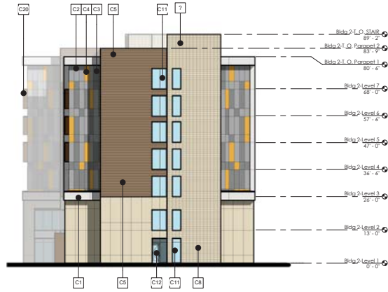
Building 2 - East Elevation (BW) 1/16" = 1'-0"
