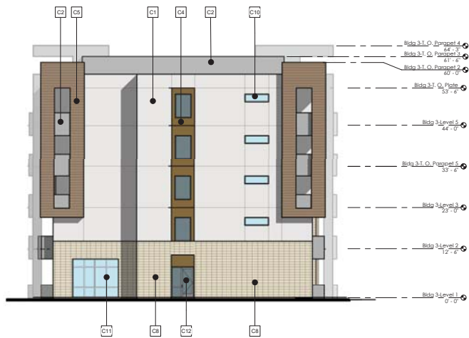
Building 3 - North Elevation - BW 3/32" = 1'-0"
