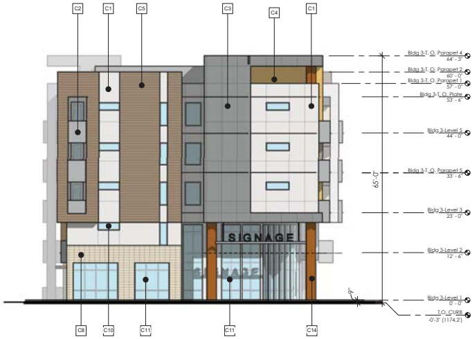
Building 3 - South Elevation (BW) 3/32" = 1'-0"
