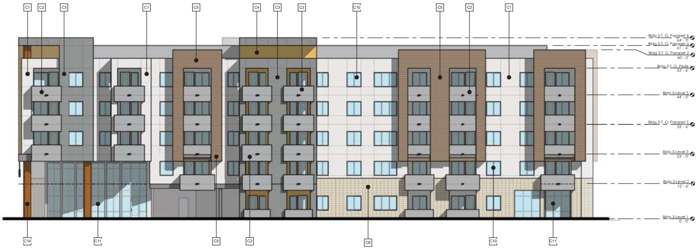
Building 3 - East Elevation (BW) 3/32" = 1'-0"
