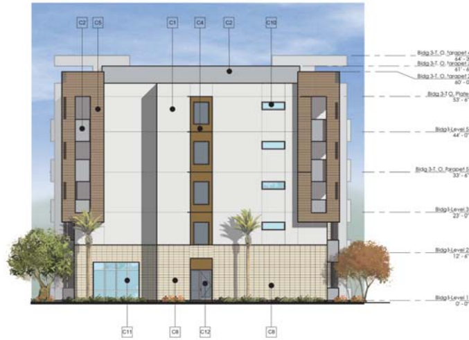
Building 3 - North Elevation 3/32" = 1'-0"
