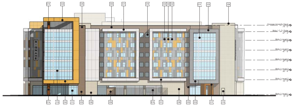
BUILDING 1 - EAST ENLARGED ELEVATION (BW) 1/16" = 1'-0"
