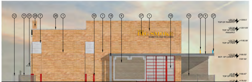
4 BUILDING C2 - EAST ELEVATION 1/8" = 1'-0"
