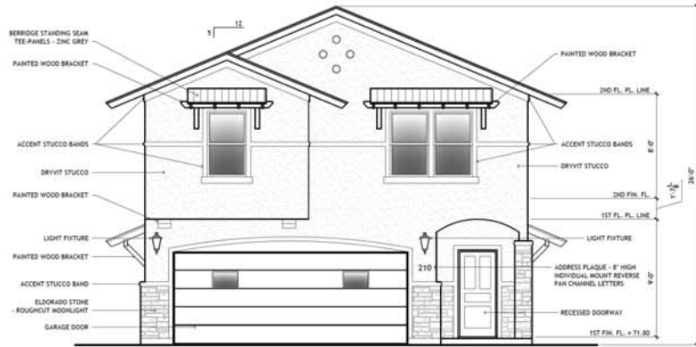
1 FRONT ELEVATION - BUILDING TYPE A 1/4" = 1'-0" • WEST ELEVATION - BUILDINGS 1 (MIRRORED) • WEST ELEVATION - BUILDINGS 2-3
