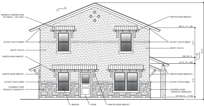
4 LEFT SIDE ELEVATION - BUILDING TYPE B 1/4" = 1'-0" + NORTH ELEVATION - BUILDING 4 + SOUTH ELEVATION - BUILDING 5
