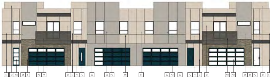
1 FRONT ELEVATION BUILDING X WEST ELEVATION SCALE 1/8"=1'-0"
