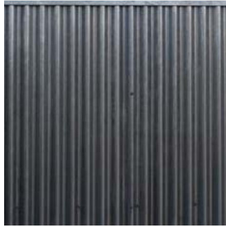
2 GALVANIZED 24 GA CORRUGATED STEEL DECK
