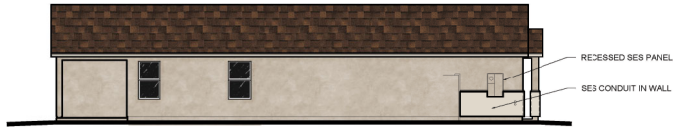
EAST ELEVATION ELEVATION A 1/8" = 1'-0"
