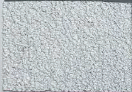
STUCCO TEXTURE - MEDIUM SAND FINISH (SAMPLE OF TEXTURE ONLY, NOT COLOR)
