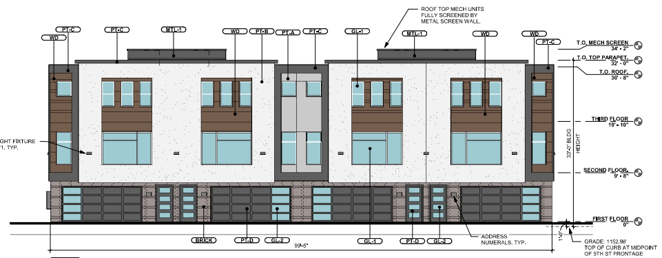
2 ELEVATION BLDG A & C EAST 1/8" = 1'-0"
