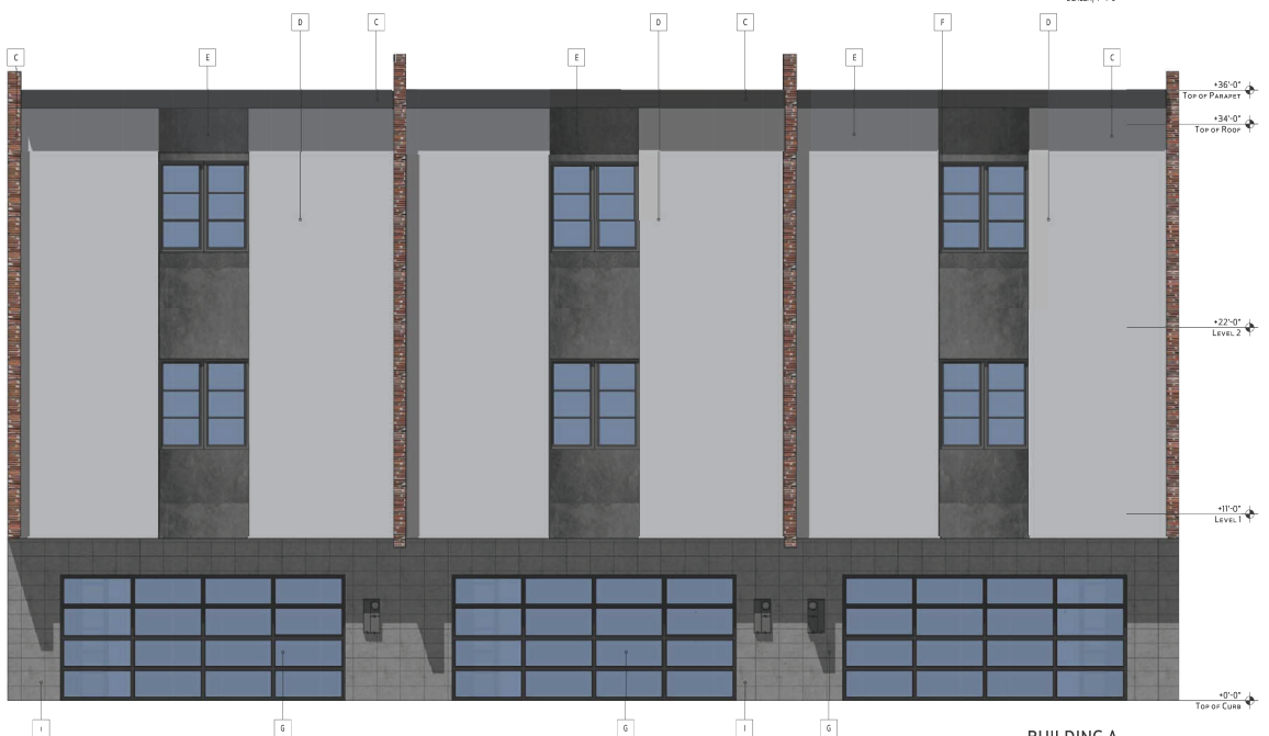
3 BUILDING A SOUTH ELEVATION SCALE: 1/4"=1'-0"
