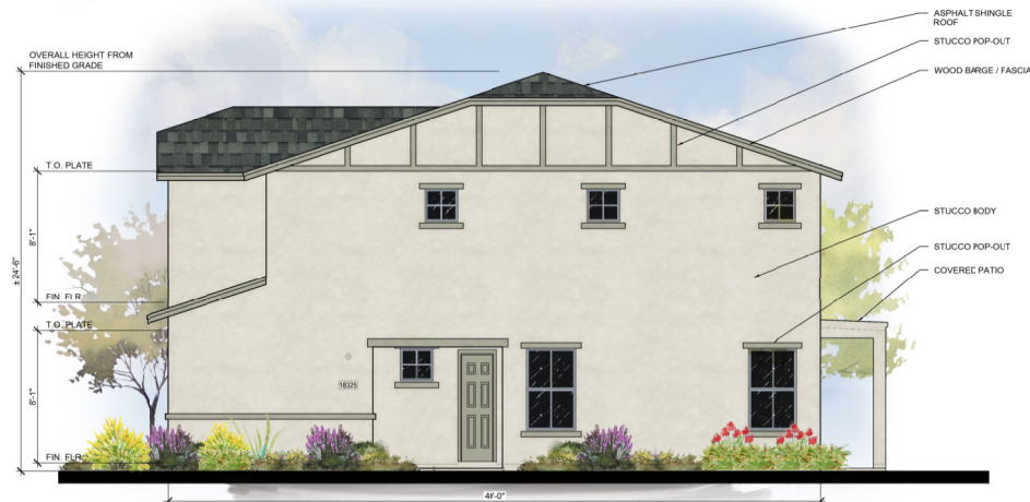
FRONT ELEVATION OPT SIDE ENTRY ELEVATION B 1/4" = 1'-0"
