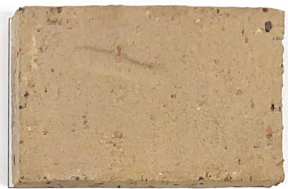
BR-1 BRICK MANUFACTURER: ACME STYLE: UTILITY SIZE: 4 X 4 X 12 COLOR: PARK AVENUE
