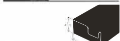
WOW-1: BLACK ANODIZED ALUMINUM WINDOW FRAME W/ 1" INSULATED GLASS W/ LOW-E COATING
