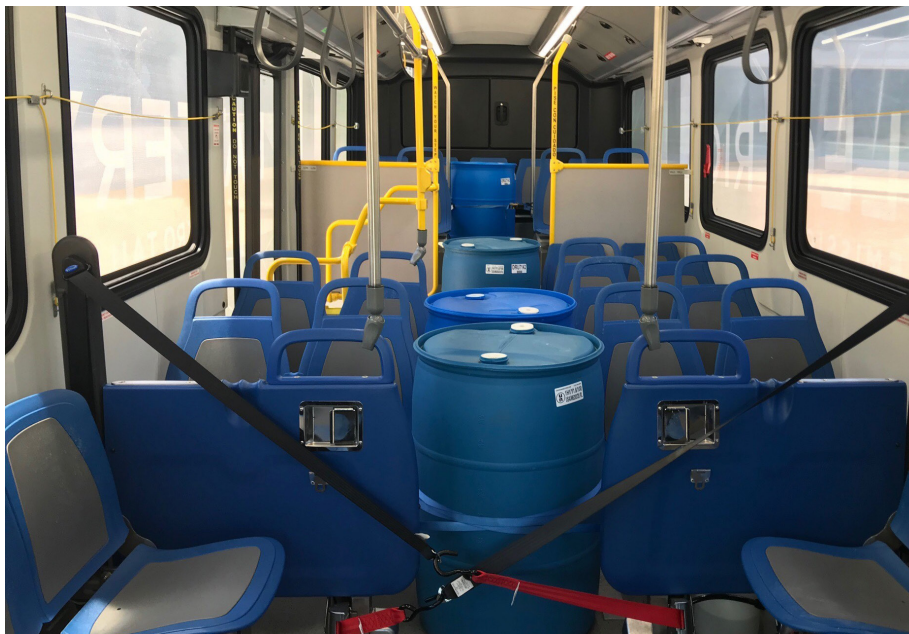
6: Interior of Proterra bus with water barrels
