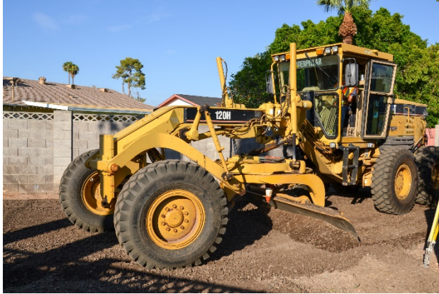
Municipal Utilities staff operating the motor grader (above left) and roller (above right), two of the pieces of equipment used to recondition alleys.
