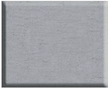
SYNTHETIC STUCCO FINISH SMOOTH SAND FINISH COLOR: MATCH EXISTING GRAY COLOR
