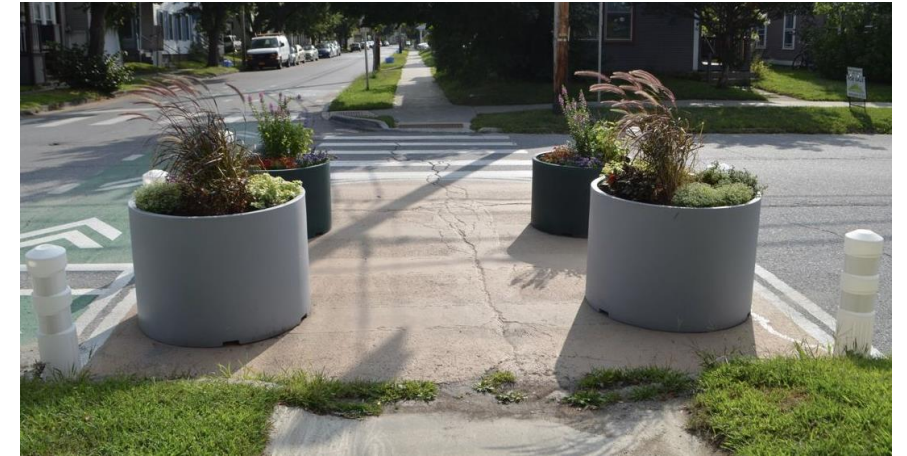
Movable planters, and other temporary vertical options to increase awareness of new intersection improvements
