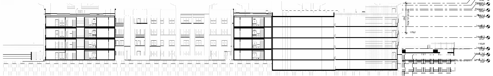
2 BUILDING SECTION E-W SCALE: 1/16" = 1'-0"
