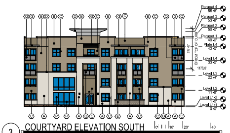
3 COURTYARD ELEVATION SOUTH SCALE: 1" = 20'-0"
